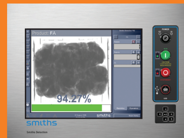
This SimulTask™ 4.0 image inspects the meat for foreign object contamination as well as CL value. The CL value of this raw trim meat (featured above) is 94.27%.
