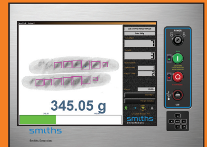
Twin pack of garlic and butter baguettes rejected for incorrect butter placement, even though the package is correct weight
